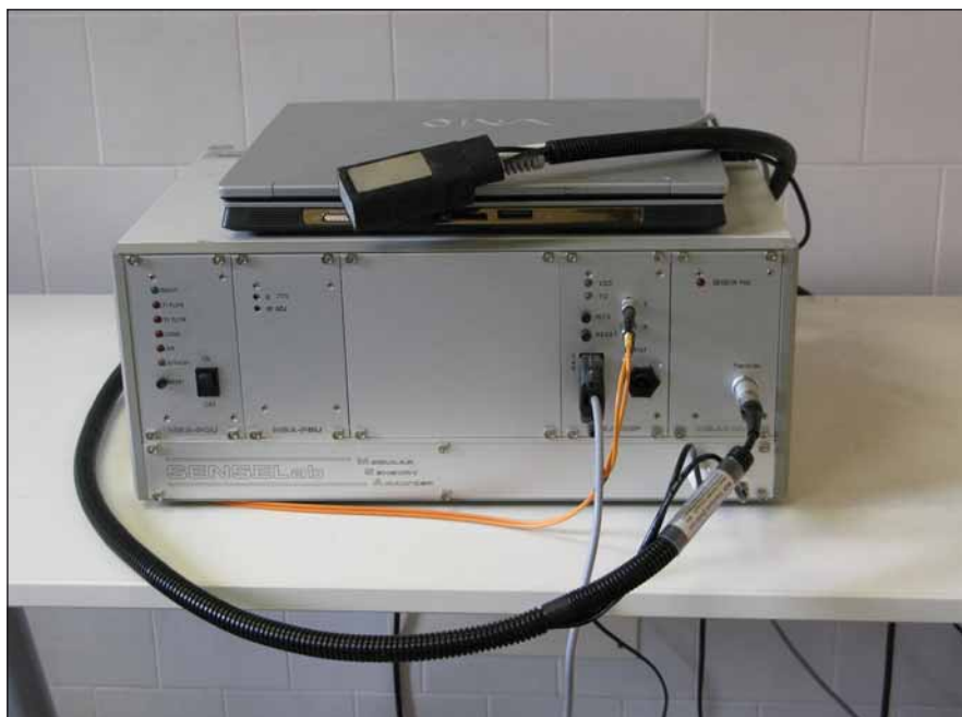
Obr. 1. Teplotní stimulator SENSELab – TERMOTEST MSA, Somic, termoda 25 × 50 mm. Fig. 1. Thermal stimulator SENSELab – TERMOTEST MSA, Somic, Thermode 25 × 50 mm.
