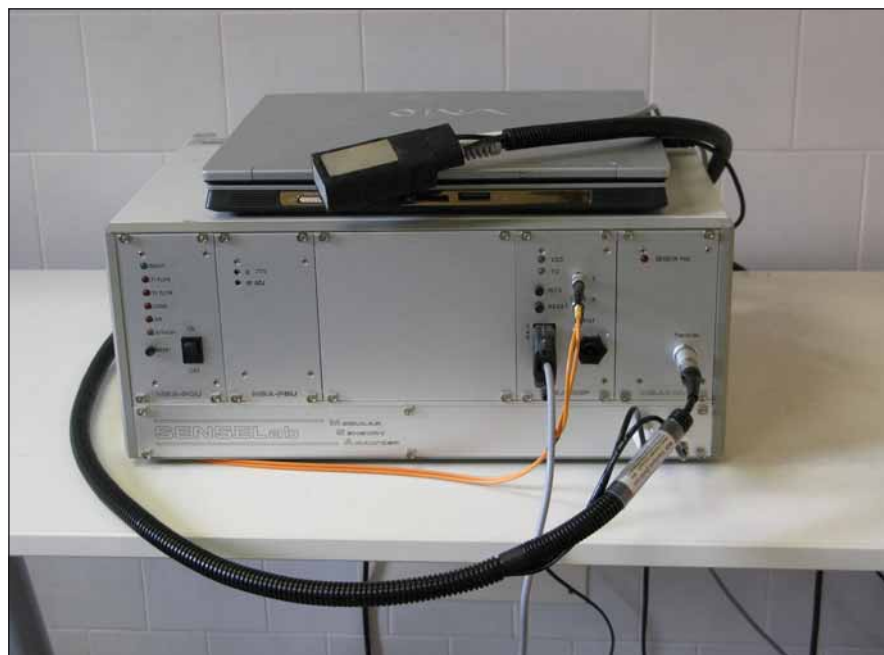
Obr. 1. Teplotní stimulator SENSELab – TERMOTEST MSA, Somedic, termoda 25 × 50 mm. Fig. 1. Thermal stimulator SENSELab – TERMOTEST MSA, Somedic, Thermode 25 × 50 mm.
